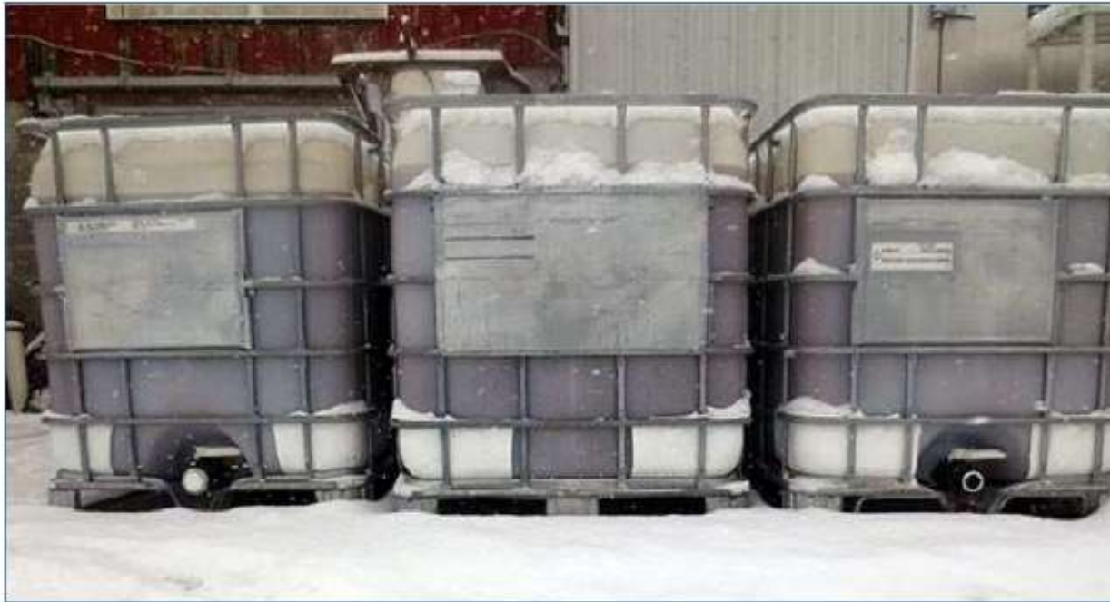
Picture 2.1: Ice cider, produced with cryo-concentration from bulk freezing, relying on outside temperatures (Picture from Eve's Cidery, 2017).
